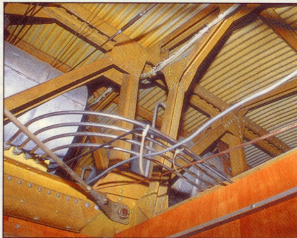
A 450-hp Pratt hangs from the wing; fairings on pylons are largely cosmetic, given the airplane's 90-mph cruise. Imagine the Bushmaster to be built like a bridge, and you'd be right.
