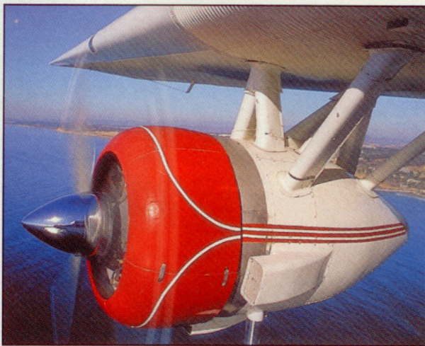
A 450-hp Pratt hangs from the wing; fairings on pylons are largely cosmetic, given the airplane's 90-mph cruise. Imagine the Bushmaster to be built like a bridge, and you'd be right.
